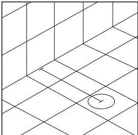
1. Prepare the waste drain hole on ceramic tiles according to closer rough in distance. Field condition is finished and clean water supply is installed.
