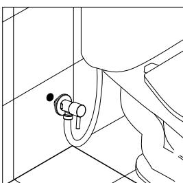
7. Install the stop valve and connect it to the water tank.
