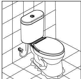
8. Apply sealant around the gap between the body and the floor.
