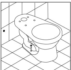
3. Install the closet body, screw firmly.
