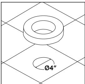
2. Place the rubber gasket on top of the waste drain hole.
