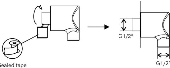
Stick the sealed tape to threaded pipe so there are no leakage
