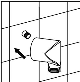
Connect the body with water inlet pipe
