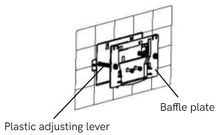
3. Insert baffle into plastic adjusting lever and tighten with screw.
