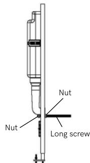
6. Adjust the length of the long screw to expose the iron support according to the thickness of the wall and fix the screw on the iron support with a nut.
