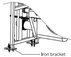
2. Fix the iron bracket to the ground.
