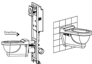
9. Insert the toilet with the small and big straight pipe into the screw rod and fix it according to the arrow direction.
