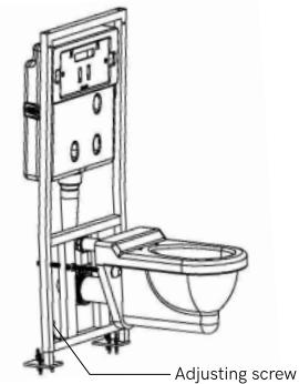
1. Adjust the iron bracket according to the height and fix it.
