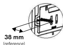
4. Adjust the distance between the plastic screw and the baffle.
