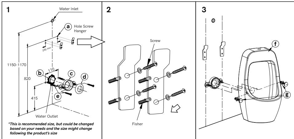
\* This illustration below is for wall hang urinal with top inlet manual flush.
