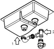
1. Put in and tighten the connector to the sink, followed by the elbow.
