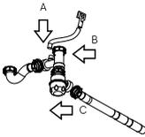
3. A. Put in and tighten the overflow pipe to the T-connector and connect it to the cup body.
