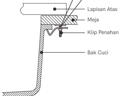
1. Insert bolt into fixing plate
