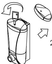
2. Rotate and pull the cap key until the dispenser cap fall out.
