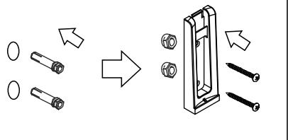
2. Position the fisher to the hole. Insert the hanger body and screw afterwards. Tighten it perfectly.
