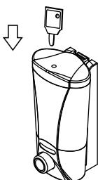
1. Use cap key and put it in the hole on the top of the dispenser cap.
