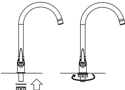
3. Insert rubber washer and cap nut to the body of the faucet. Tighten it perfectly.
