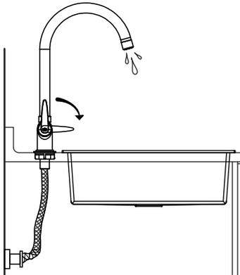
5. Rotate the handle 90° to turn the water on and check whether there are any problems or leakage.
