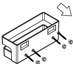
3. Position the body to the fisher assembly. Put in and tighten the screw to the body.
