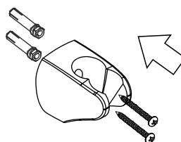
Position the fisher to the hole, followed by hanger and tighten with screw.
