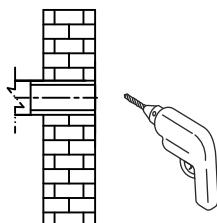
Make a hole according to the fisher size.
