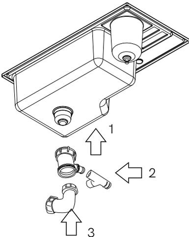
2. 1. Put in and tighten the connector to the sink.
