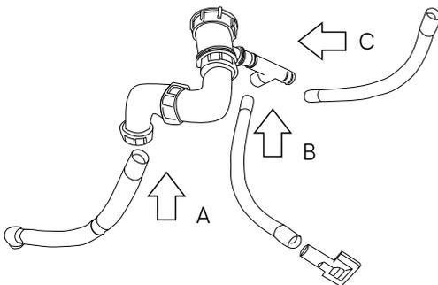
3. A. Put in and tighten the outlet pipe to the elbows.
