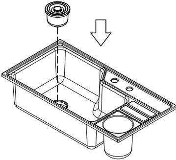
1. Put in and tighten the cup body to sink.
