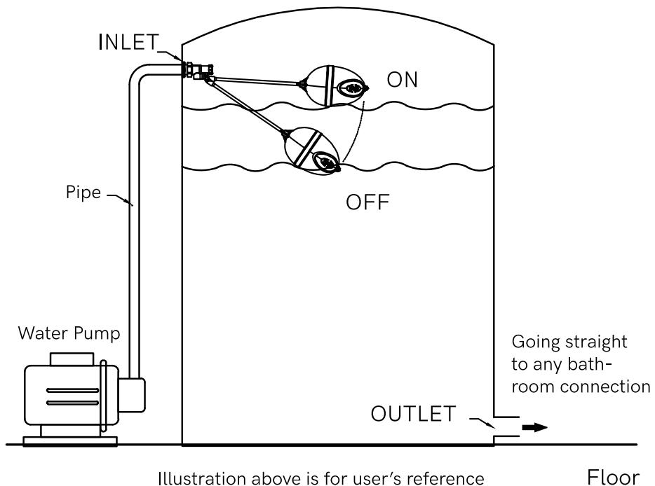
\* This installation instruction is suitable for floating valve with diameter 1/2", 3/4" and 1"
