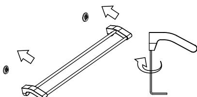
4. Position the towel bar to the hole. Tighten the body with the assembly by using allen key.
