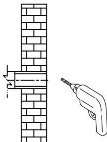
1. Make hole in the wall and make sure that the diameter is suitable for the fisher.
