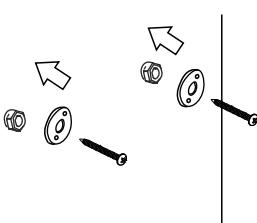
3. Insert the seal and screw afterwards. Tighten it perfectly.
