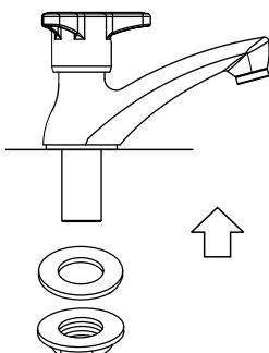
3. Insert rubber washer and cap nut to the body of the faucet.
