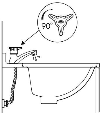
5. Rotate the handle  $90^\circ$  to turn on the water and turn it back to turn the water off.
