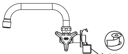
② Stick the sealed tape to threaded pipe so there are no leakage
