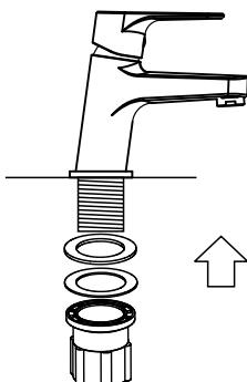
3. Insert rubber washer, clamp, and nut to the body of the faucet. Tighten it perfectly.
