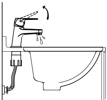
5. Raise the handle up to turn the water on and check whether there are any problems or leakage.
